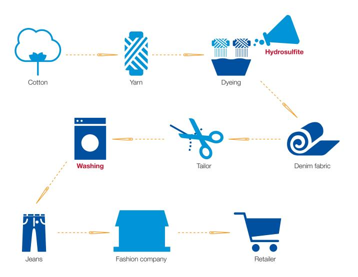
The quality of Hydrosulfite is one of the most important factors for denim manufacturers because faults in denim dyeing are difficult to detect until the very last moment – i.e. when the jeans have been produced. This means that denim quality largely depends on the quality of the Hydrosulfite reducing agent and indigo used.
