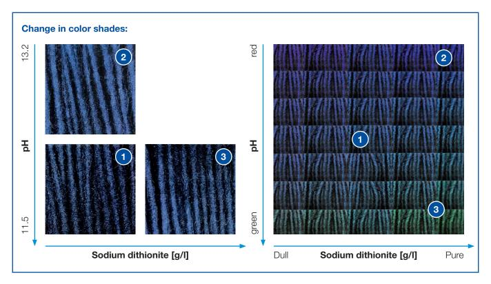
The indigo-dyed yarn may appear more greenish, reddish, dull, or pure depending on the ratio of sodium dithionite and caustic soda. The smallest variation in terms of sodium dithionite content can affect dyeing results, such as ring dyeing, fastness, and color fixation. Thanks to the stable sodium dithionite content in HydroBlue®90, consistent dyeing results are ensured in order to reproduce the same shade.
