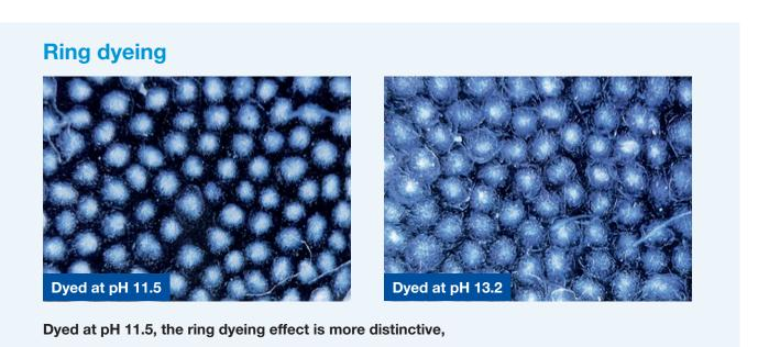
compared to pH 13.2 where greater dye penetration is visible.
